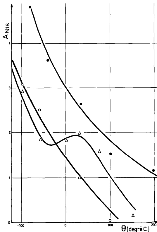
FIG. 3. NO and NO 2 adsorption isobars (1 Torr) obtained with Fe 2 O 3 and Fe 3 O 4 : (Δ) NO on Fe 3 O 4 ; (○) NO 2 on Fe 3 O 4 ; (●) NO 2 on Fe 2 O 3 .
